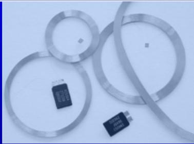
A photograph showing several circular and oval-shaped metal loops of varying sizes, which are the antennas for low-frequency RFID tags. Two small black integrated circuits are also visible on a white surface.                        |
